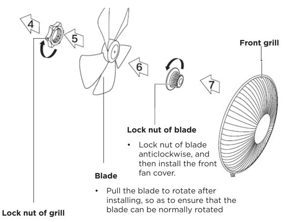
• Screw the lock nut of grill clockwise to secure the rear grill.
