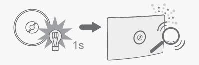
Flashing light: Hub is updating its software or is searching for receivers.
