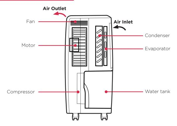
This product is a dehumidifier. It controls relative humidity by passing the air through the unit, forcing the excess moisture to condensate over the cooling elements. Contact with this cold surface causes the moisture in the air to condense. This condensed water then drains safely into the water tank. The dried air then passes through the condenser where it is slightly warmed and re-enters the room at a slightly elevated temperature.
