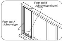
1. Cut the adhesive foam seal A and B strips to the proper lengths, and attach them to the window sash and frame as shown.
