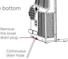
• When the water level of the bottom tray reaches a predetermined level, the unit will beep 8 times and the digital display area will show "P1". At this time the air conditioning/dehumidification process will immediately stop. However, the fan motor will continue to operate (this is normal). Carefully move the unit to a drain location, remove the bottom drain plug and let the water drain away. Reinstall the bottom drain plug and restart the machine. If the error repeats, call for service.
