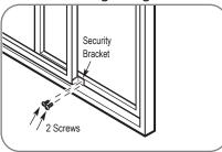
4. If desired, install the security bracket with 2 screws as shown.
