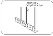
3. Cut the non-adhesive foam seal C strip to match the width(or height) of the window. Insert the seal between the glass and the window frame to prevent air and insects from getting into the room.
