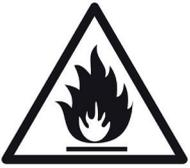
**WARNING:** For using R290 refrigerant. This symbol shows that this appliance uses a flammable refrigerant. If the refrigerant is leaked and exposed to an external ignition source, there is a risk of fire.
